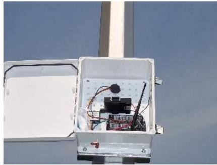
The wireless CR206 data logger is mounted on a street lamp pole at 15 feet above the ground for security purposes.
