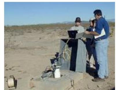
*Training on the operation of the miniTROLL water level logger at Monitoring Well #1*
