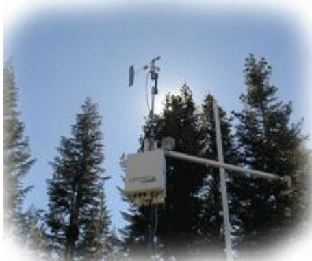
The upper monitoring site includes sensors for measurement of wind speed and direction, temperature and relative humidity, and snow depth
