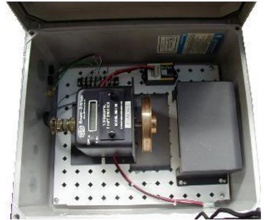
*Close-up of Shaft Encoder, power supply and regulator inside enclosure that is mounted on stilling well.*
