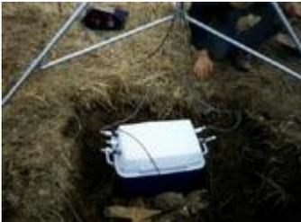
*Plastic cooler instrument vault is prepared for burial.*
