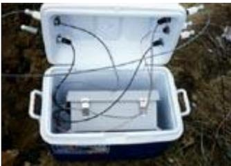
*Enclosure is sealed inside of a plastic cooler, to protect it from vandalism.*
