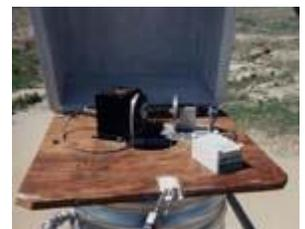
*Pond 212 site close up of Shaft Encoder and Aqua Pod Water Level Logger installed on the stilling well.*
