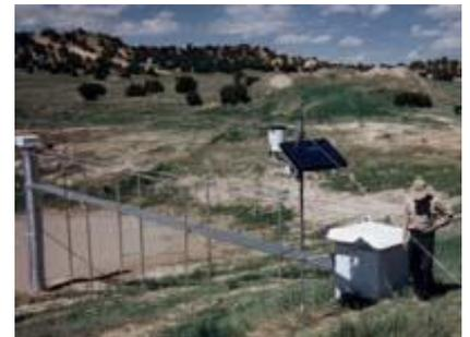
*Pond 212 site with Precipitation Gauge, Temperature Sensor, and a Shaft Encoder attached to a CR10X data logger.*
