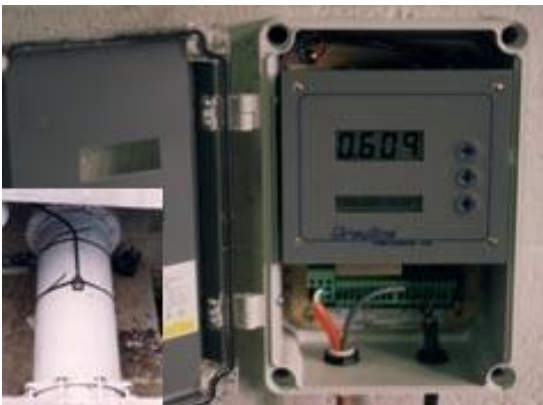
Greyline DFM-III Closed Pipe Flow Monitor. (Inset) Doppler Ultrasonic sensor strapped to pipe.
