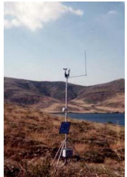
*A weather Station at Skinner Lake: Measuring Air Temperature, Relative Humidity, Wind Speed & Direction, Soil Moisture, Soil Temperature, and Precipitation with a Handar 555 data logger.*
