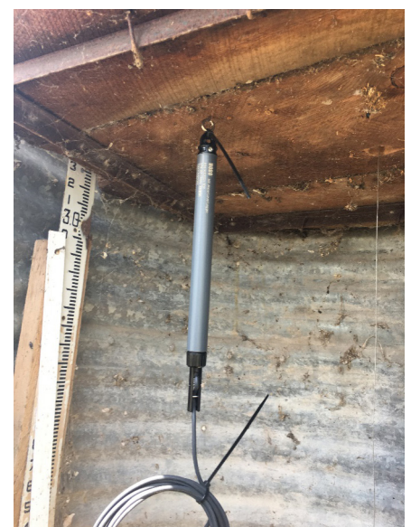
MX2001 shown fastened to the underside of the wooden shelf in a stilling well
