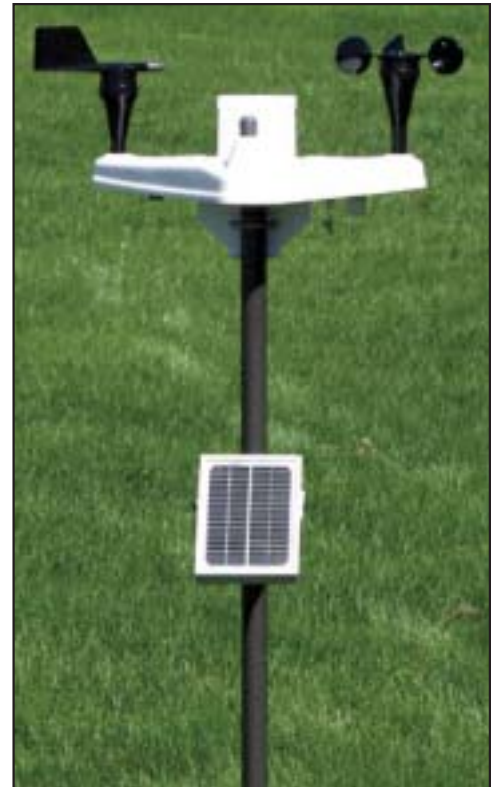
WeatherHawk provides real-time weather measurements and calculates ET_0 on an hourly and daily basis.
