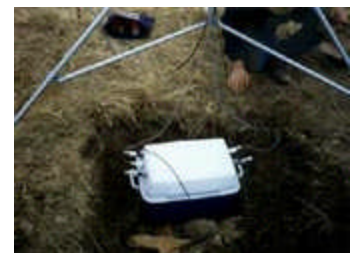
Plastic cooler instrument vault is prepared for burial.
