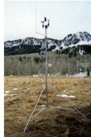
Weather Station near Park City, Utah. Data logger is buried to protect it from vandalism and the environment.
