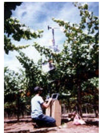
Greg McCurdy performs final calibration and testing on weather station at Far Niente vineyard.
