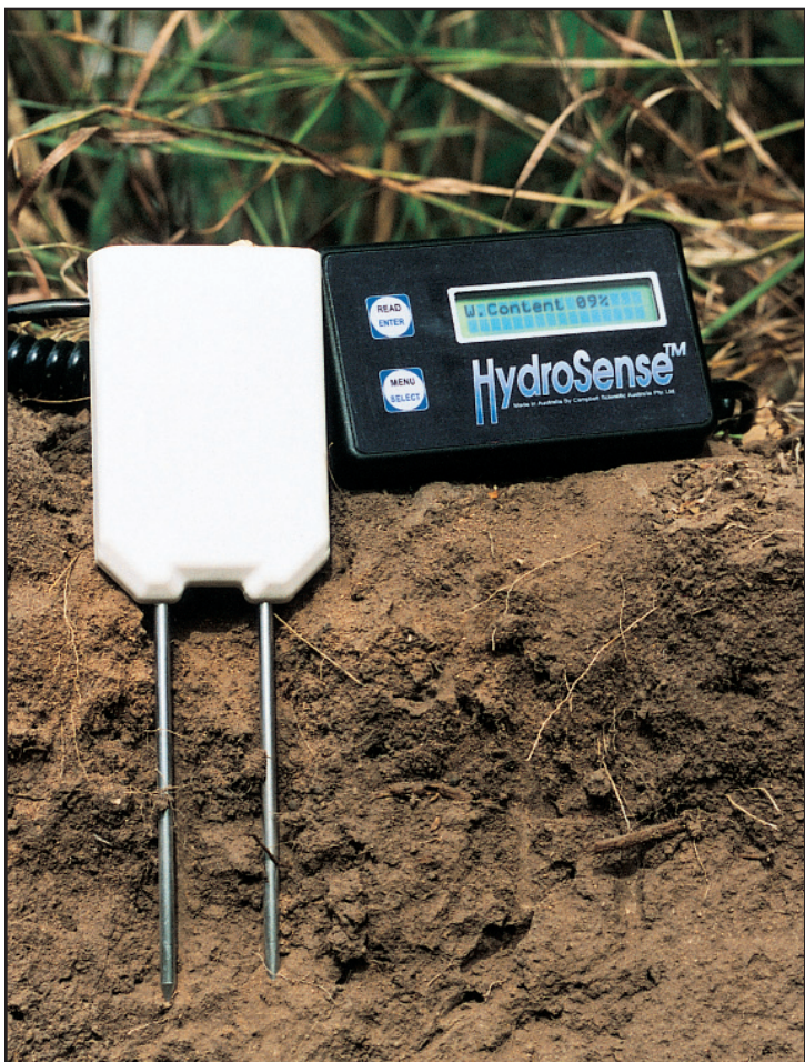
The HydroSense system consists of the CS620 sensor (left) and the CD620 display (right).
